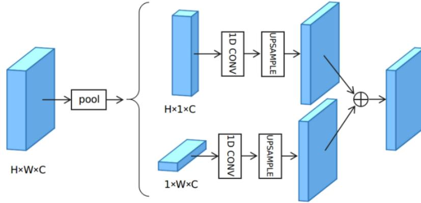
Figure 4. The structure of Branch2 in CMSI, which uses strip pooling to capture long-distance features.
