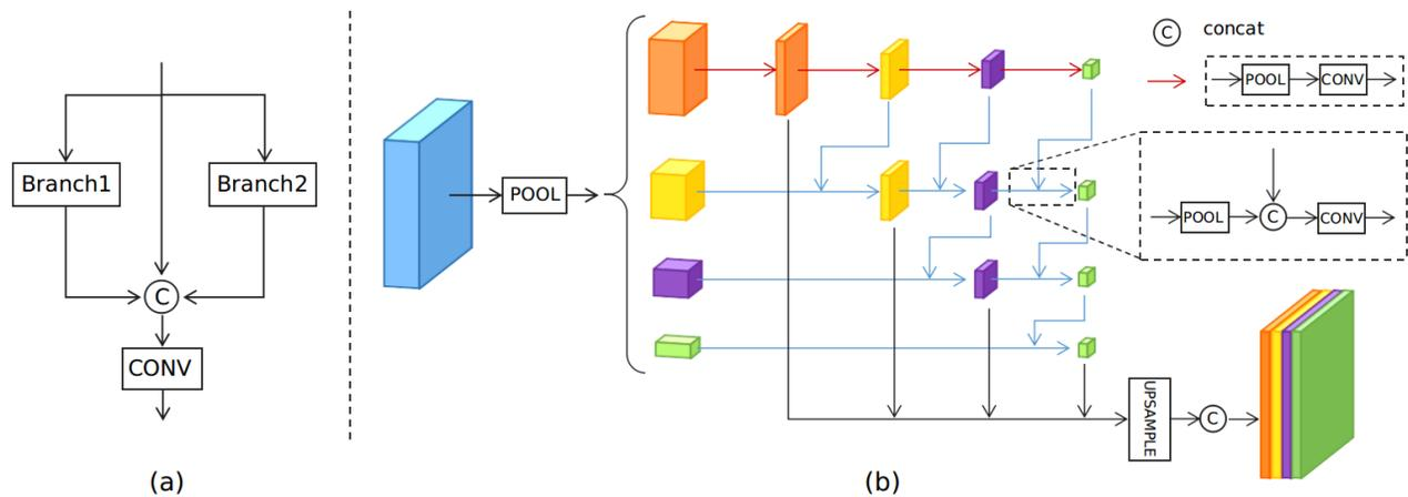
Figure 3. (a) The structure of the proposed CMSI module. (b) The structure of Branch1 in CMSI, which uses cascaded pooling and convolution to interact with different scale features.
